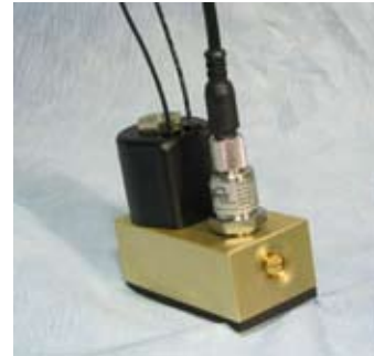
600 PSI manifold assembly with pressure transducer and test solenoid valve, 4000 PSI burst pressure, individually tested at 1000 PSI. Available on FM and CE controllers only. UL Listed controllers available with 290 PSI maximum rating.
