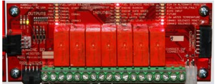
Engine Relay Board for field engine connections including ECM engines and PLD engines
