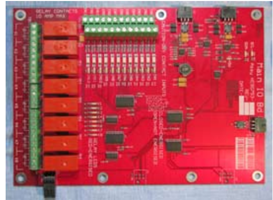
Main I/O board with terminals for field connection of pump house alarm inputs and alarm output contacts
